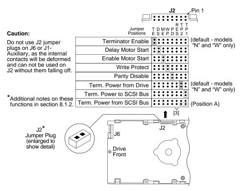
Figure 11. Hawk 4XL family drive option select header for models "N" and "W"
