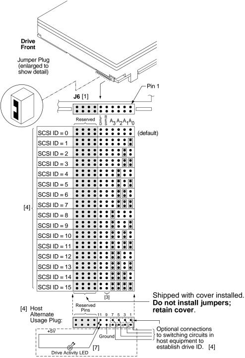
[4] Dashed area is optional host circuitry (external to the drive) connected to host supplied optional usage plug. Do not connect anything to pins 13-20.
