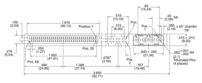
Figure 17. Non-shielded 68 pin SCSI device connector used on "W" model drives
