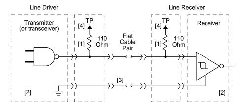
Figure 18. Single-ended transmitters and receivers
