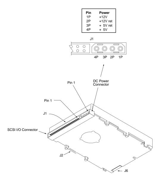
Figure 13. Physical interface for "N" model drives
