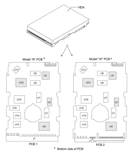
Figure 4. Locations of printed circuit board (PCB) components listed in Table 3
