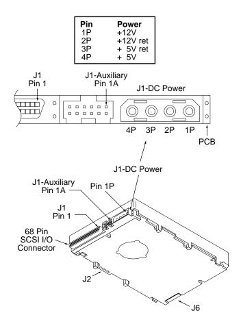
Figure 14. Physical interface for "W" model drives
