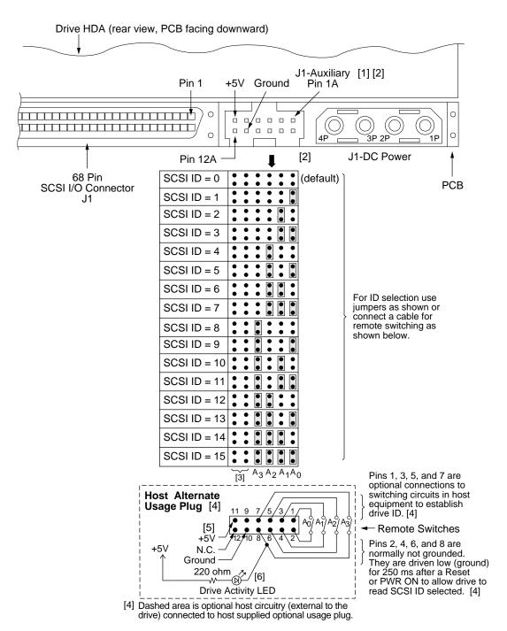
Figure 10. Hawk 4XL family drive ID select header J1-auxiliary for model "W" (J1-Auxiliary Pins 1A - 12A)
